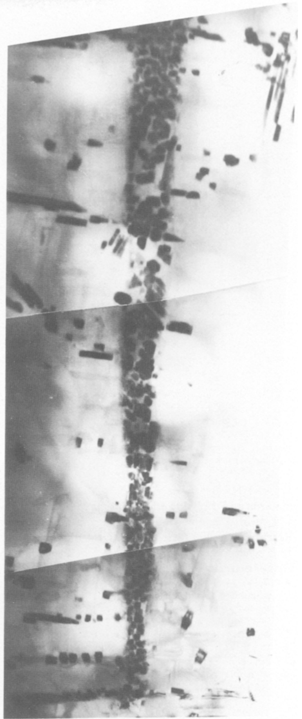
Figure 9 As Fig. 8, tilted to show carbide precipitation ( M_{23}C_6 -type) associated with the stacking fault. Note also the faceted features of the precipitate.
